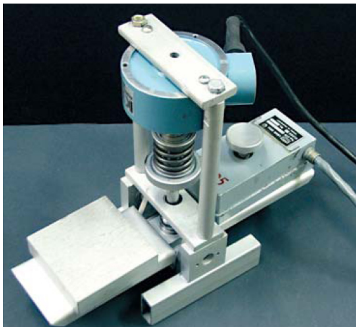
The Zwick Roell GZM 10-K is a universal testing machine used for lubricity examination.
